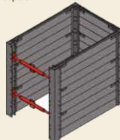
Install spreaders at required locations (see tabulated data).
