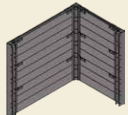
Install lift-eyes then 2nd and 3rd corner post.
